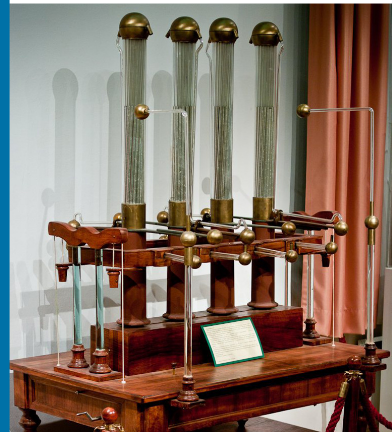
Jedlik's impulse generator, an early predecessor of the Marx impulse generator
